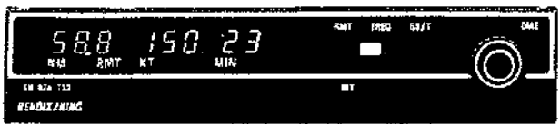
Figure 3. Distance/Groundspeed/TTS. RMT mode.
