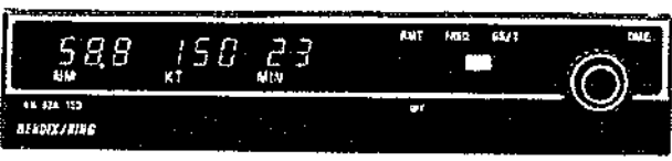
Figure 2. Distance/Groundspeed/TTS. GS/T mode.
